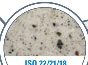
ISO 22/21/18 Typical cleanliness of delivery
