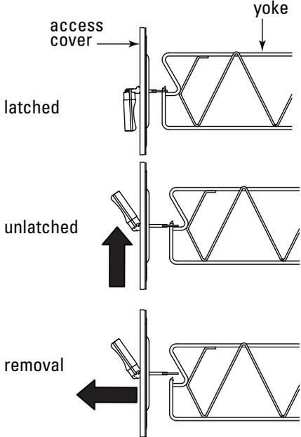
Optional and Bag-In/Bag-Out Filter Access Cover Removal (Top View)
