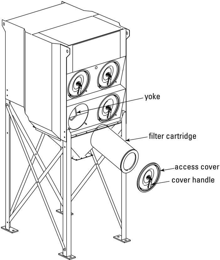
Filter Access Cover Removal (Side View)
