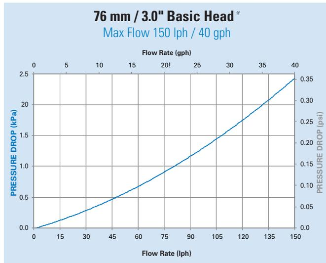
\* Filter elements add an additional 1-2 kPa (0.14 - 0.29 psi) restriction to filter assembly at the max recommended flow rate.
