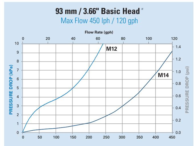
\* Filter elements add an additional 1-2 kPa (0.14 - 0.29 psi) restriction to filter assembly at the max recommended flow rate.
