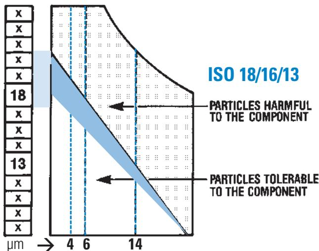
Fluid analysis and field monitoring are the only ways to get these measurements. Combine data from several tests to form a range of performance. Remember, actual filter performance will vary between applications.
