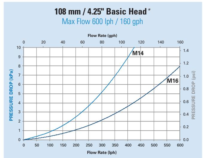
\* Filter elements add an additional 1-2 kPa (0.14 - 0.29 psi) restriction to filter assembly at the max recommended flow rate.
