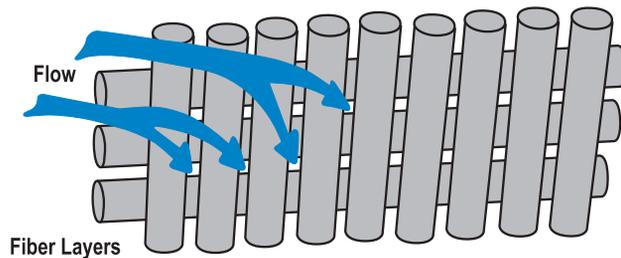
The fluid changes direction as it comes into contact with the media fibers, as illustrated above. As the fluid flows through the media, it changes direction continuously as it works its way through the maze of media fibers. As it works its way through the depths of the layers of fibers, the fluid becomes cleaner and cleaner. Generally, the thicker the media, the greater the dirt-holding capacity it has.
