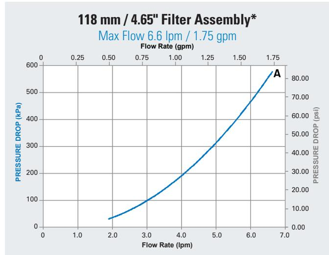
\*These performance curves represent clean filter by-pass flow as a function of system pressure.
