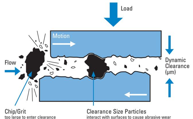
The circuit actually generates additional particles as the fluid comes into contact with the precision machined surfaces of cylinder walls and pistons, injector needles and pistons and crankshaft bearings. Contaminant levels can keep doubling with every new particle generated. The result can be catastrophic if these contaminants are not properly filtered out of the system.
