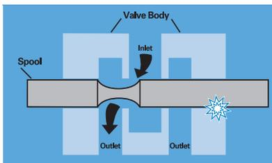
This cutaway view of a simple oil valve illustrates how particles damage components. In normal operation, the spool slides
