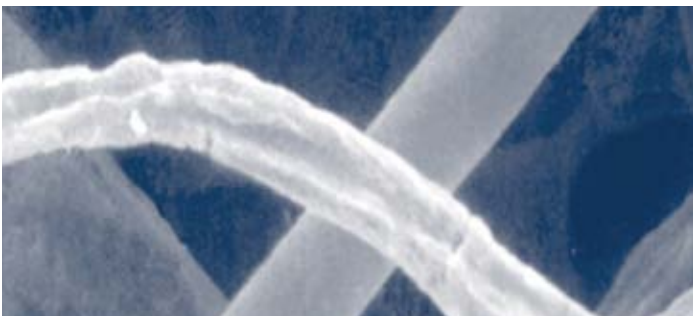
Commodity Filter Media (600px) – Conventional media has spaces of up to 60 µm between fibers, allowing dust to become deeply embedded.
